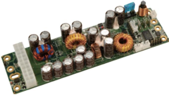
**Dedicated ATX Power for Car PC and Battery Powered Applications**
